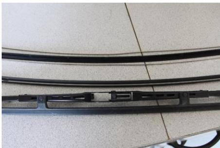
The picture at left shows the old blade removed (top) and the new blade (middle), with the holder at the bottom.
