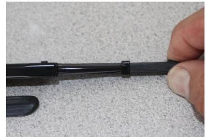
separate from the rubber blade). To install the wiper refill, insert it from the bottom and feed it through all the retainers until you get past the top one, and which time you'll have to push firmly on the bottom to get it to seat/lock in place.
