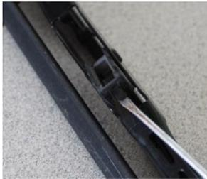
The easiest way to start is to remove the holder from the arm. To do this (with or without hood open), you simply push up on the retainer tab and slide the holder back (see picture at left). To replace the blade, simply grab the blade on the sides at the bottom edge (this would be the edge on the right as looking at the blade in its parked position), and pull. You have to give a good tug, and will slide right out. As you pull the blade out, it may come apart (i.e., the two metal runners
